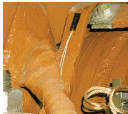
BLUE PETER Series® flexible surface sensors work very well here in monitoring DC Field Coil temperatures.
